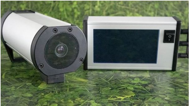
Figure 3. The Clovercam System by Agpointelli. A high-resolution RGB-camera and a processing terminal, displaying the current legume proportion.
